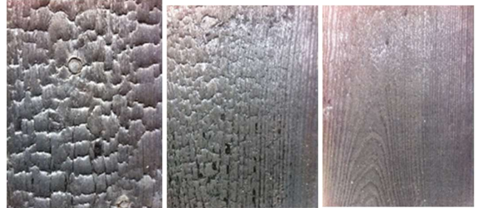
Fig 7 Shou Sugi Ban test panels
